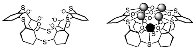
Fig. 7. Schematic drawing of \text{tca}[6]^{6-} in pinched-cone conformation (left) and formation of penta-nuclear cluster in the cavity of \text{tca}[6]^{6-} (right); tert -butyl groups have been omitted.
